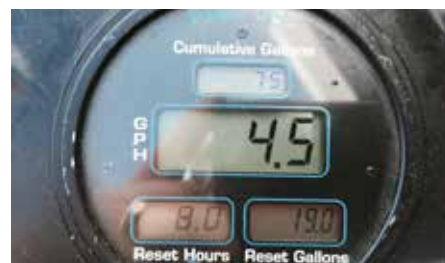
Approximately the same readings using a FLOWSCAN meter installed in the fuel lines of the generator.
