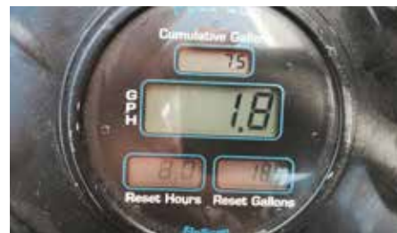
Approximately the same readings using a FLOWSCAN meter installed in the fuel lines of the generator.
